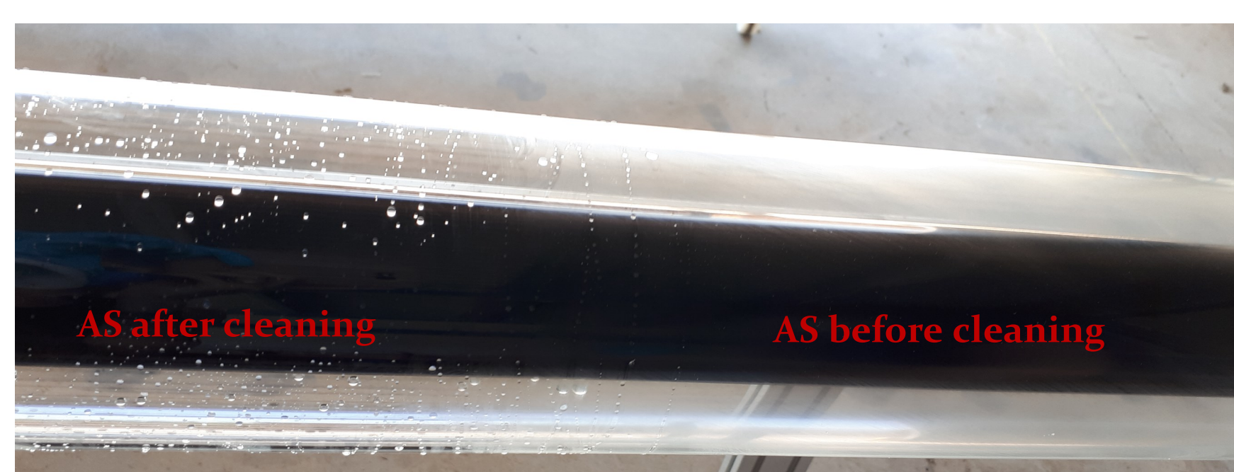
Fig. 1. Picture of a glass receiver tube coated with the AS solution before cleaning (right) and after cleaning with DI water (left)
