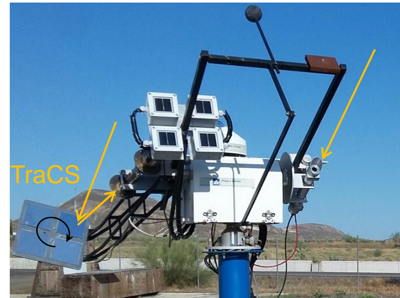
Tracking Cleanliness Sensor – TraCS - working principle
